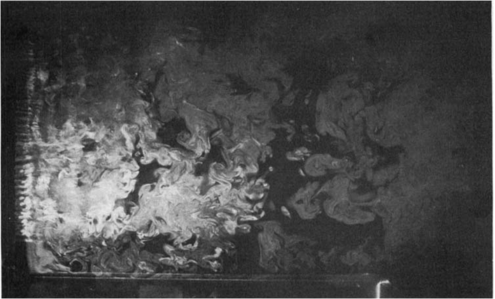
FIGURE 3. Smoke photographs of the separated shear layer in the (x, z) -plane 32 mm above the splitter plate ( Re_{\eta_F} = 1.5 \times 10^3 ).
